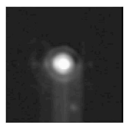
11.7 micron image of the comet and a standard star (alpha Boo). The FWHM of the standard is 1.1 arcsec and that of the comet is 1.8 arcsec. Therefore the extended coma was detected.
