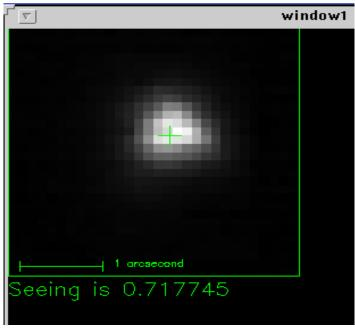
This seeing values provide by the Gaussian fit algorithm should be recorded in the trouble log.
