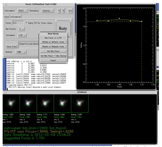
Window1 shows the seeing measurement (white) and the Fit (yellow) Window 2 shows the sub images with it's seeing and focus values. The POLYFIT results, time stamp, and suggested focus is displayed.
