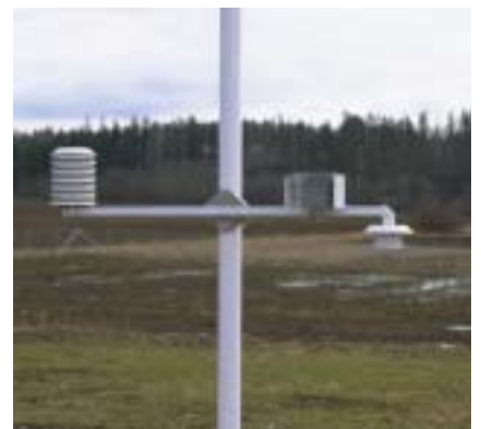
HMP243MIK provides radiation shields for dewpoint and temperature sensor heads.
