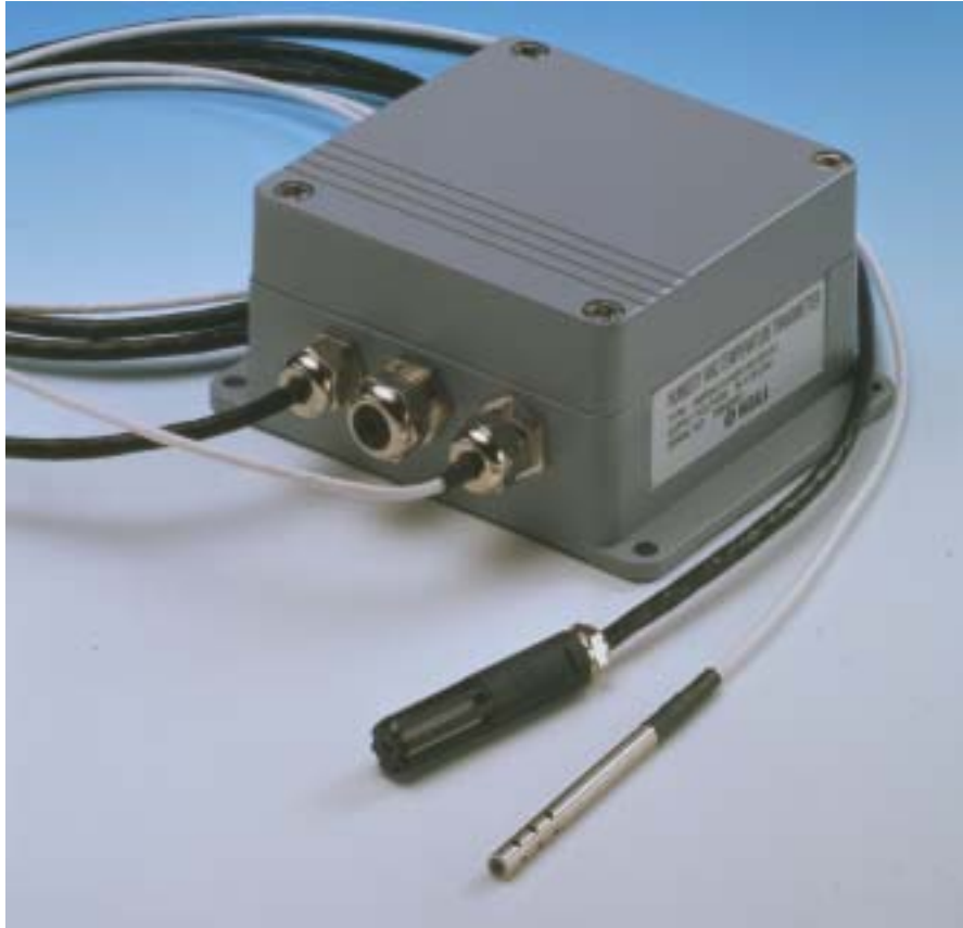
The HMP243 Transmitter, shown with a PPS plastic grid, non-condensing humidity sensor and optional temperature sensor, typically needs calibration/maintenance once a year.
