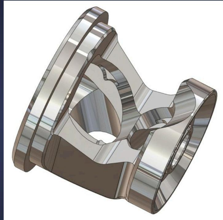
Note: The middle mirror of the K-mirror assembly is separated from the main hub because it would be very difficult to fabricate as one part.
