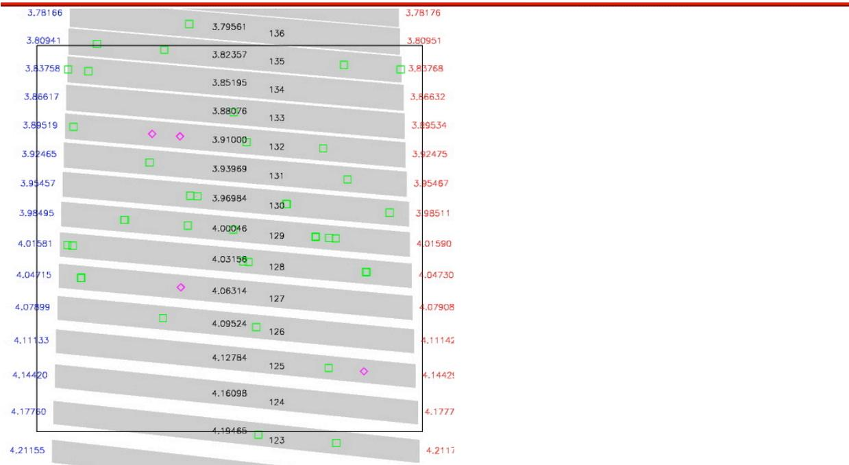
**Figure 35. XD setup for long slit observation of  $H_3^+$  in Jupiter,  $L'$  order sorter ( $R=72,000$ ,  $0.38 \times 25''$  slit, XD  $3.7 \mu\text{m}$  blaze at  $42.0$  degree). The highest priority orders are 126-132 ( $3.9$ - $4.1 \mu\text{m}$ ).**
