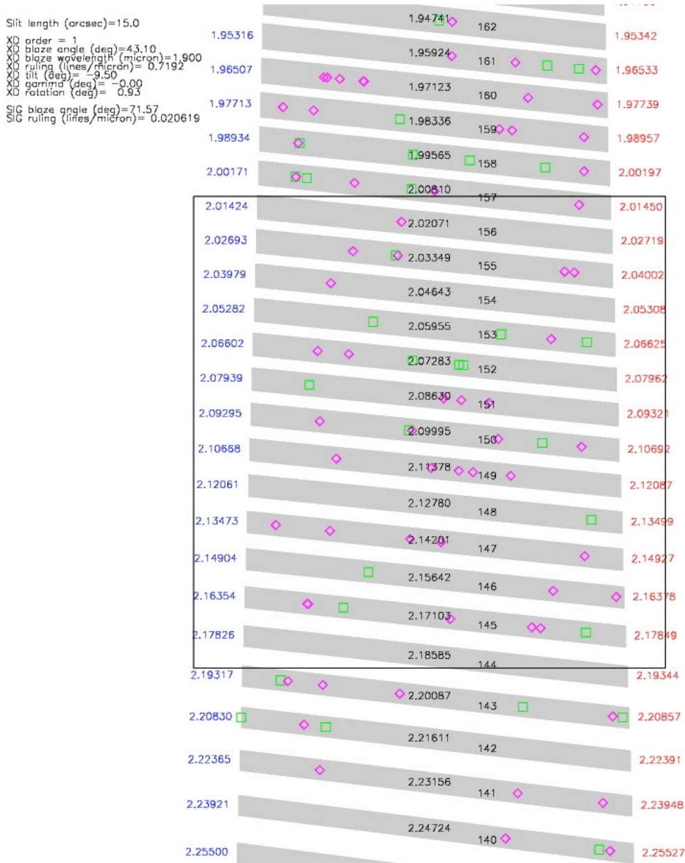
Figure 10. Exposure K2 (see Table 5), slit length 15", 720 line per mm grating. The box indicates the H2RG array.
