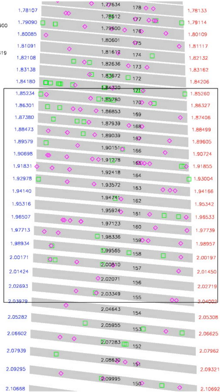
Figure 9. Exposure K1 (see Table 5), slit length 15", 720 line per mm grating. The box indicates the H2RG array.
