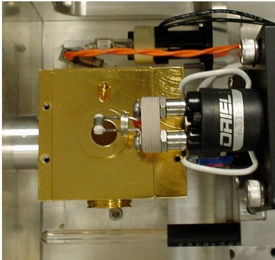
**Figure 24. SpeX integrating sphere showing QTH lamps (top), IR lamps (middle), argon arc lamp (bottom), positioned in front of their respective input ports.**
