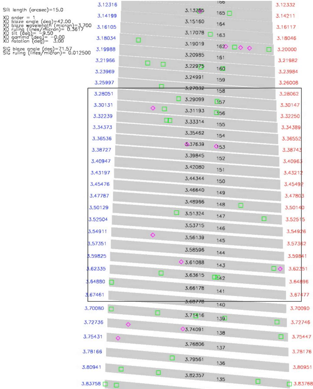
Figure 16. Exposure L4 (see Table 5), slit length 15", 360 line per mm grating. The short wavelength limit (about 3.28  $\mu\text{m}$ ) is set by the need to keep orders separated by at least 10 pixels. The box indicates the H2RG array.
