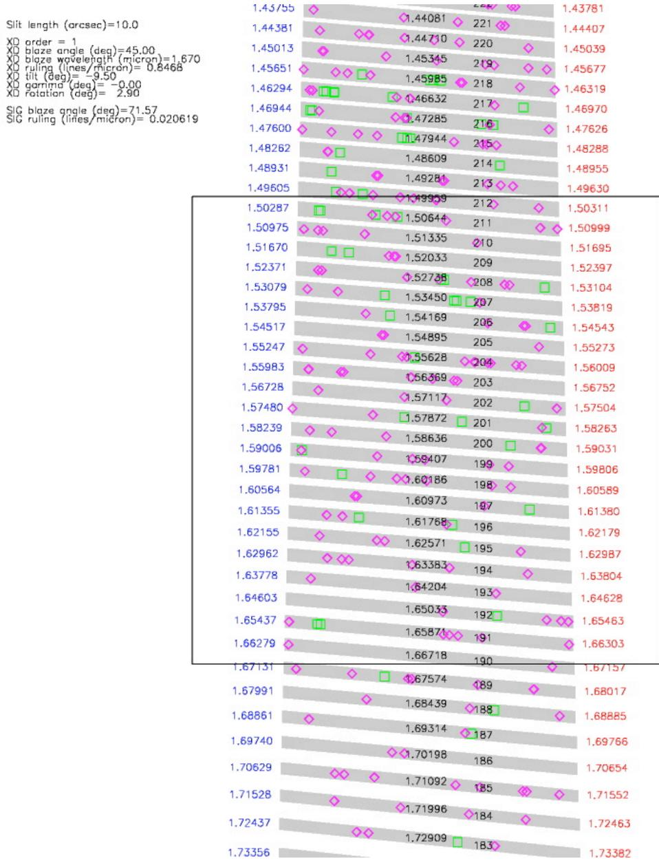
Figure 6. Exposure H1 (see Table 5), slit length 10", 847 line per mm grating. The box indicates the H2RG array.
