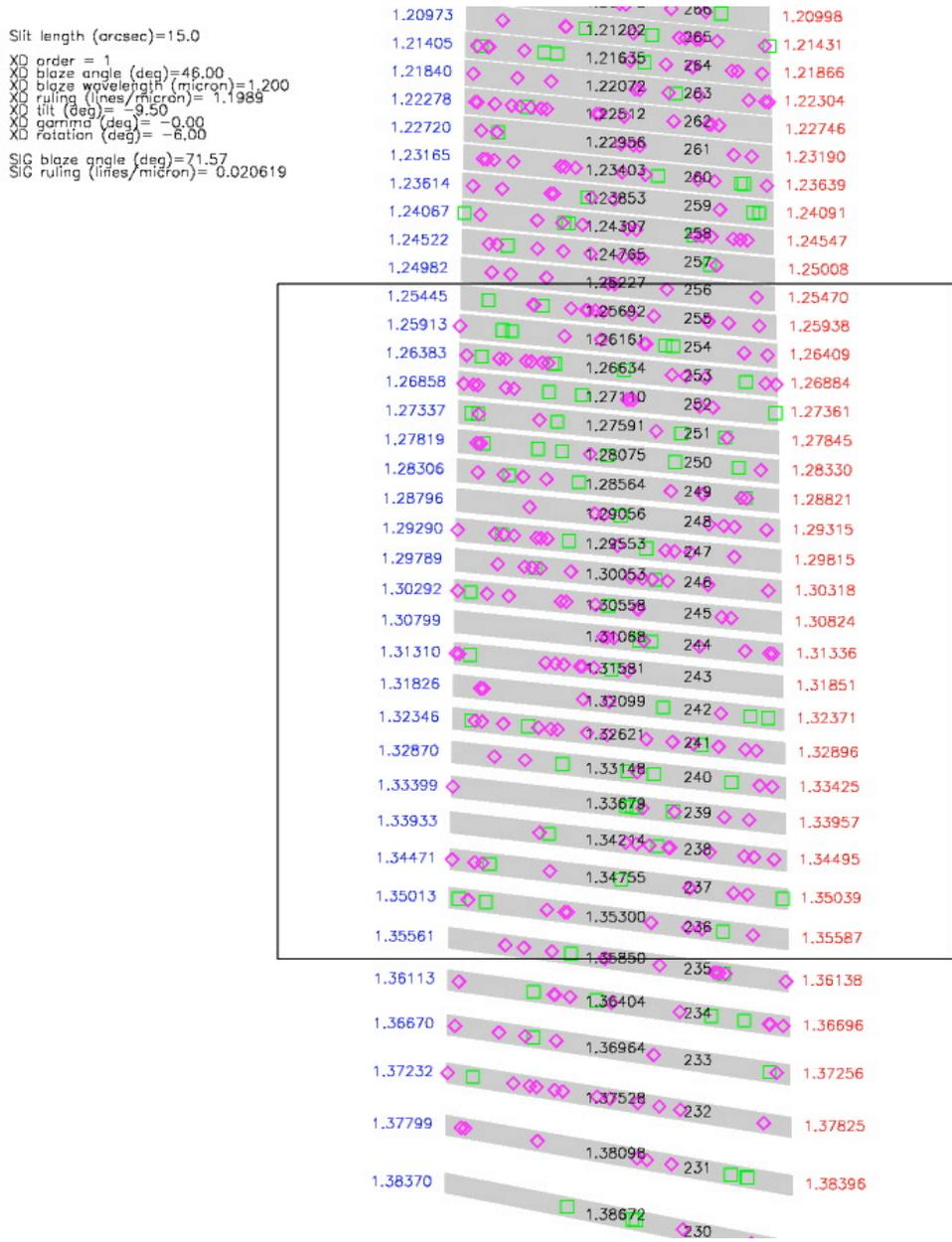
Figure 5. Exposure J2 (see Table 5), slit length 15", 1200 line per mm grating. The box indicates the H2RG array.
