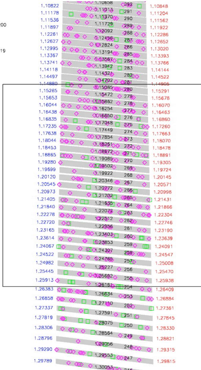
Figure 4. Exposure J1 (see Table 5), slit length 10", 1200 line per mm grating. The FSR of each spectral order is plotted. The short wavelength limit (about 1.15  $\mu\text{m}$ ) is set by the need to keep orders separated by at least 10 pixels. A box indicates the H2RG array. Symbols indicate the position of argon (green square) and thorium (purple diamond) arc lamp lines.
