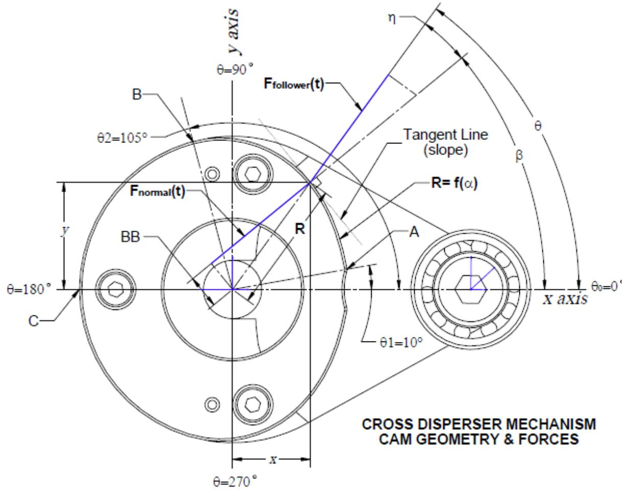
This calculation uses a sinusoidal cam follower path for a smooth transition between the seated to unseated positions of the detent mechanism.
