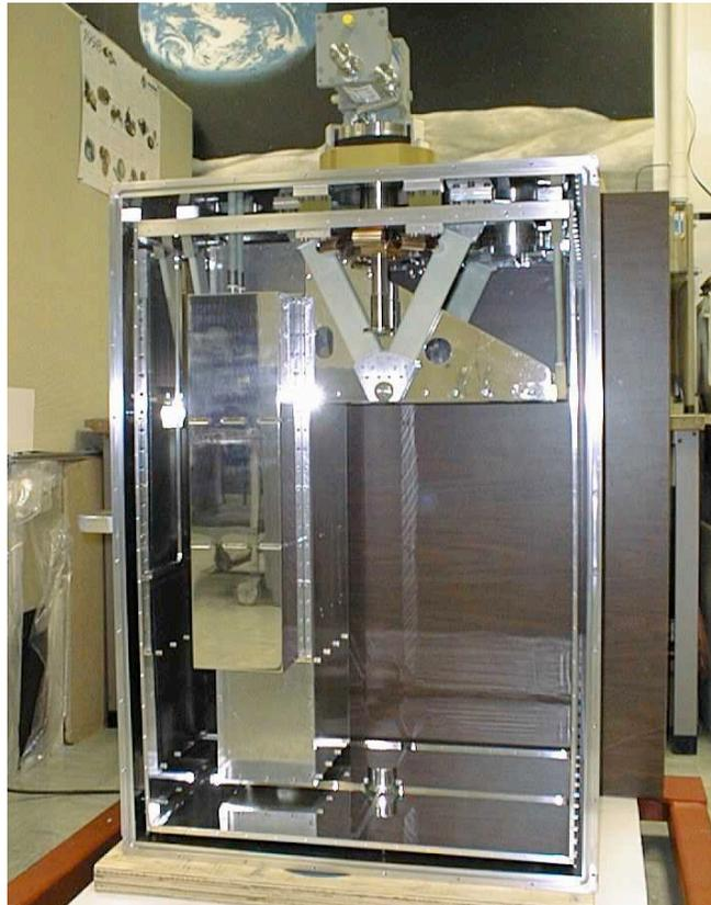
**Figure 10. The cryostat showing the vacuum jacket, cryocooler, active radiation shield (partial), liquid nitrogen can mounted to the spectrograph box, and support trusses. The fore-optics box is not installed.**
