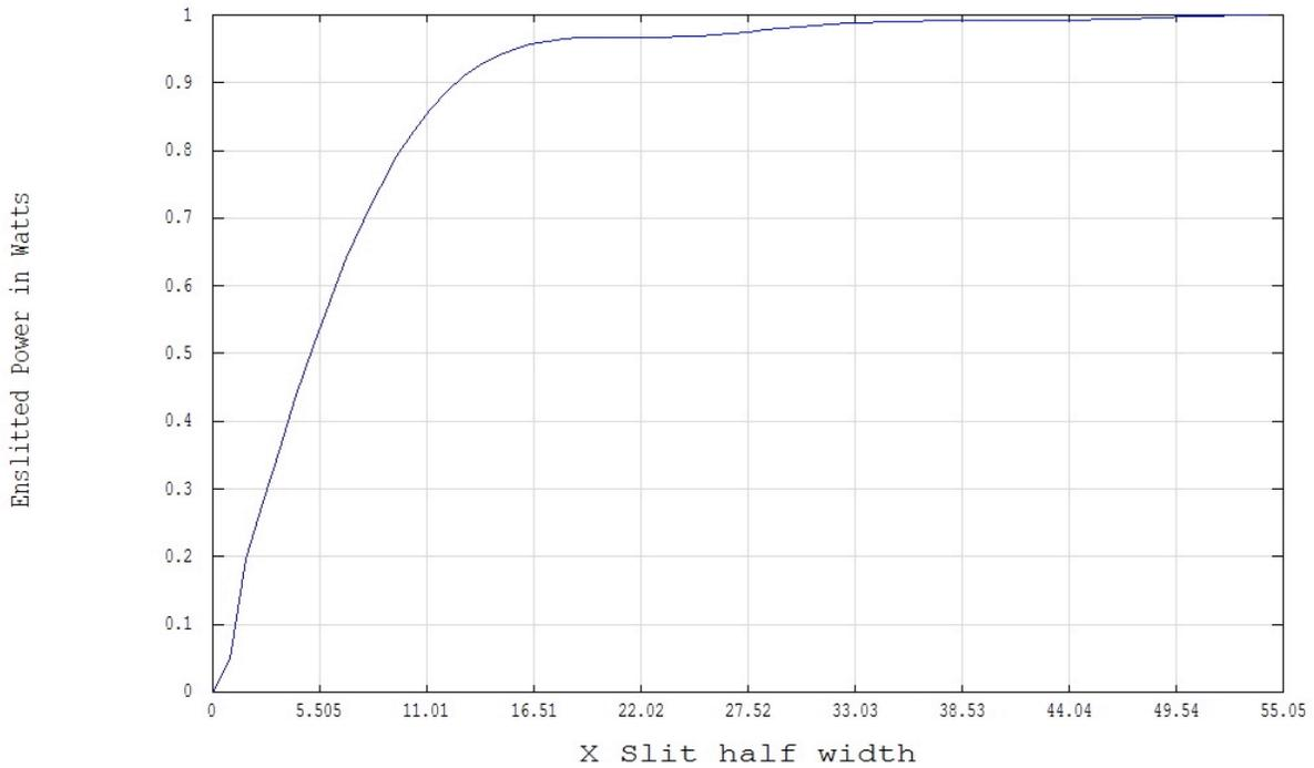
**Figure 3. Image of the telescope pupil at 4.8  $\mu\text{m}$  (including the primary hole) with the slit wide open (*top*). Enslitted energy (*bottom*). All the energy is contained within the geometrical diameter of 22.0 mm. The total intensity has been normalized to one watt.**
