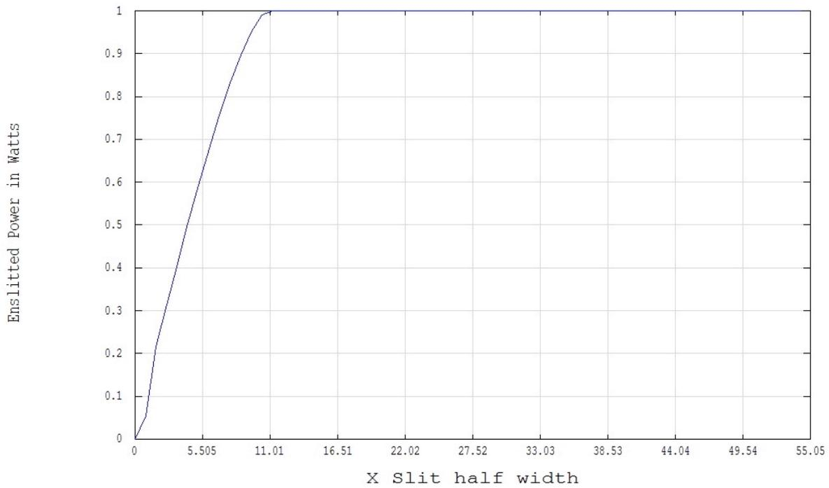
**Figure 2. Image of the telescope pupil at 4.8  $\mu\text{m}$  (including the primary hole) with the slit wide open (*top*). Enslitted energy (*bottom*). All the energy is contained within the geometrical diameter of 22.0 mm. The total intensity has been normalized to one watt.**
