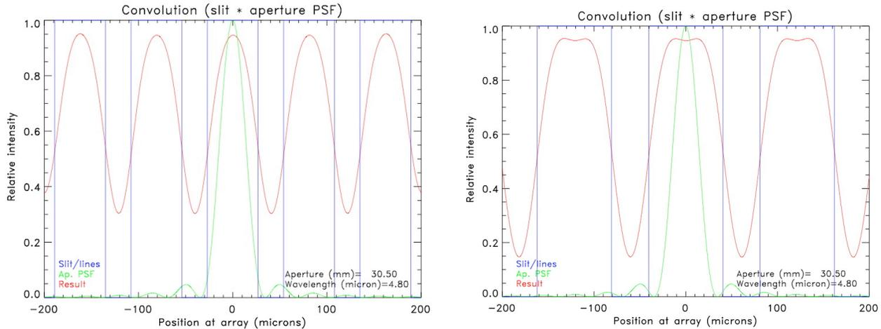
**Figure 10. (Left) Feature contrast at  $4.8\mu\text{m}$  with  $R=80,000$  matched to 3 pixels. (Right) Feature contrast at  $4.8\mu\text{m}$  with  $R=80,000$  matched to 4.5 pixels. The contrast improves from 0.5 to 0.8.**
