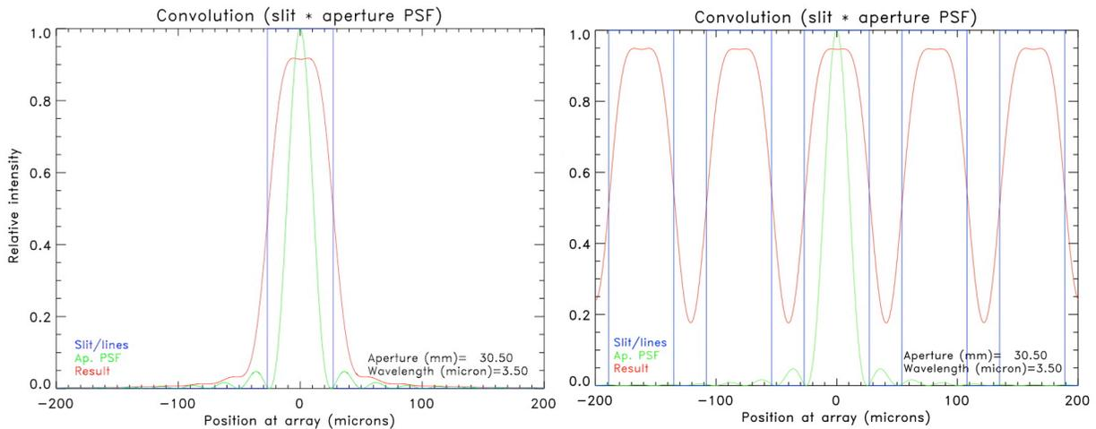
**Figure 7. (Left) The instrument profile at 3.5  $\mu\text{m}$ . (Right) With spectral features separated by half a slit width (equivalent to  $R=53,333$ ) the feature/line contrast is degraded to 0.75 (red) from the perfect instrument profile of 1.0 (blue) due to diffraction at the immersion grating aperture of 30.5 mm x 35.0 mm (green).**
