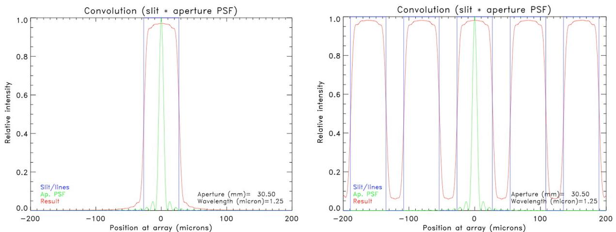
**Figure 9. (Left)** The instrument profile at 1.25  $\mu\text{m}$ . **(Right)** With spectral features separated by half a slit width (equivalent to  $R=53,333$ ) the feature/line contrast is degraded to 0.9 (red) from the perfect instrument profile of 1.0 (blue) due to diffraction at the immersion grating aperture of 30.5 mm x 35.0 mm (green).
