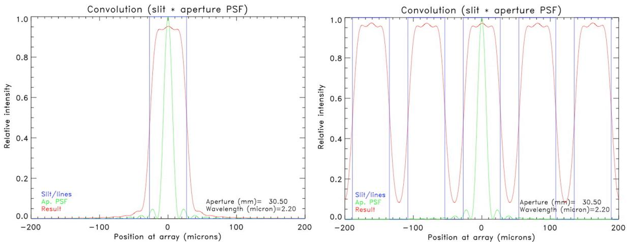
**Figure 8. (Left)** The instrument profile at 2.2  $\mu\text{m}$ . **(Right)** With spectral features separated by half a slit width (equivalent to  $R=53,333$ ) the feature/line contrast is degraded to 0.85 (red) from the perfect instrument profile of 1.0 (blue) due to diffraction at the immersion grating aperture of 30.5 mm x 35.0 mm (green).
