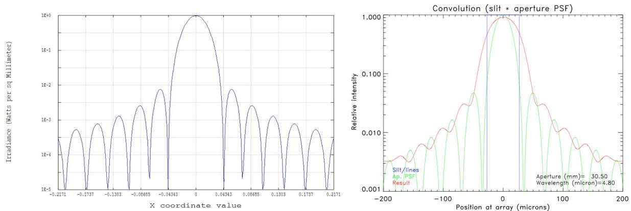
**Figure 5. (Left) The intensity profile in the dispersion direction (x in mm at the array) plotted from Figure 4 (right). (Right) The calculated instrument profile from Equation 1 (x in microns at the array). The FWHM of both profiles is the same and equal to the FWHM of the re-imaged slit onto the array, however the calculation indicated that slightly more flux is scattered into the wings of the instrument profile.**
