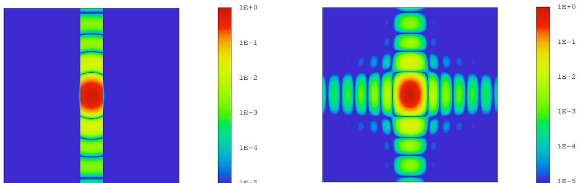
**Figure 4.** (Left) 4.8  $\mu\text{m}$  image of the slit at the array with a star focused onto the slit and with a large aperture at the pupil/immersion grating. The slit image is perfect. The Airy pattern of the star along the slit is due to diffraction of the telescope. (Right) Same image but now with the aperture at the pupil/immersion grating reduced to a 30.5 mm x 35.0 mm rectangle (immersion grating face). Diffraction at this aperture leads to the spreading of the instrument profile.
