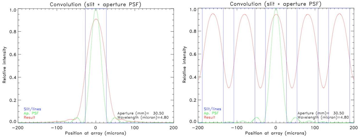
**Figure 6. (Left) The instrument profile at 4.8  $\mu\text{m}$ . (Right) With spectral features separated by half a slit width (equivalent to  $R=53,333$ ) the feature/line contrast is degraded to 0.5 (red) from the perfect instrument profile of 1.0 (blue) due to diffraction at the immersion grating aperture of 30.5 mm x 35.0 mm (green).**
