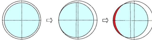
The result can be approximated fairly accurately by simply shifting the line in the above plots to reflect the fact that no effect will take place until the pupil from the secondary decenters enough to reach the side of the undersized cold stop. Plots with a 2% reduced area and a 5% reduced area are given below.
