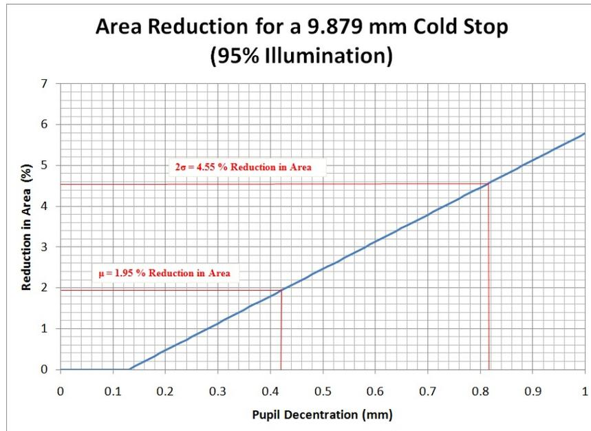
As can be seen in the chart above - by reducing the cold stop diameter to 9.879 mm (i.e. reducing the cold stop area by 5%), the variations in illumination reduce to:
