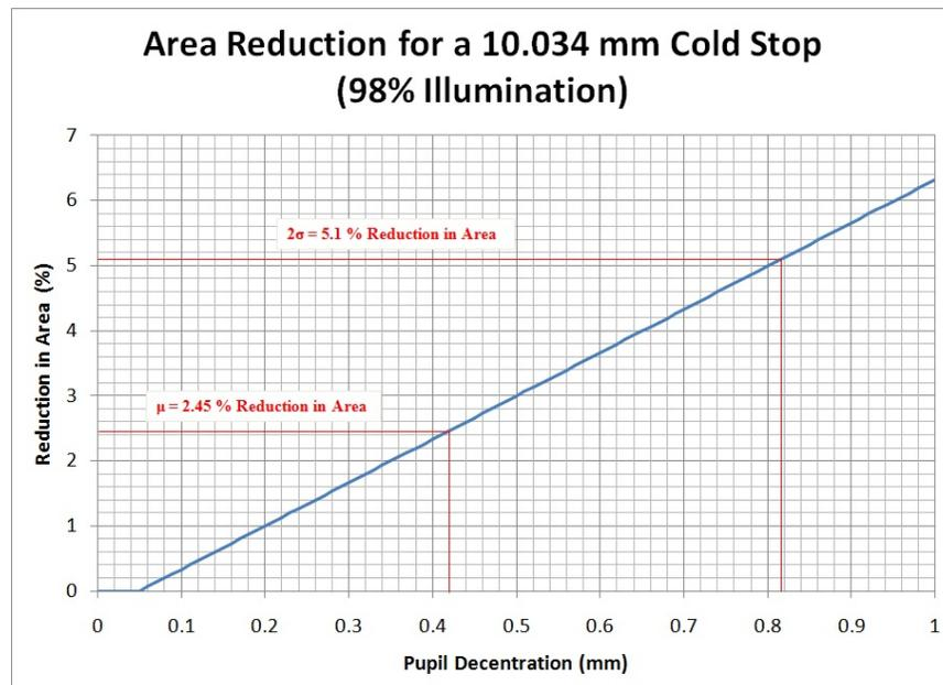
As can be seen in the chart above - by reducing the cold stop diameter to 10.034 mm (i.e. reducing the cold stop area by 2%), the variations in illumination reduce to:
