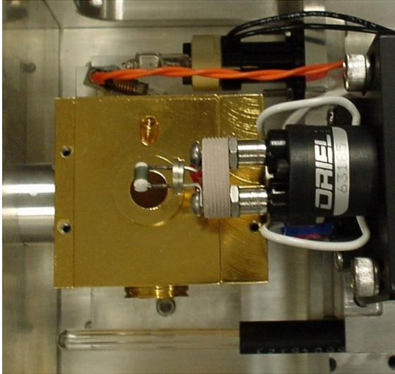
**Figure 5. SpeX integrating sphere showing QTH lamps (top), IR lamps middle), argon arc lamp (bottom), positioned in front of their respective input ports.**
