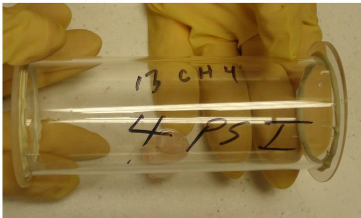
**Figure 2. The methane gas cell used in CSHELL. The cell is 150 mm long and 50 mm diameter.**
