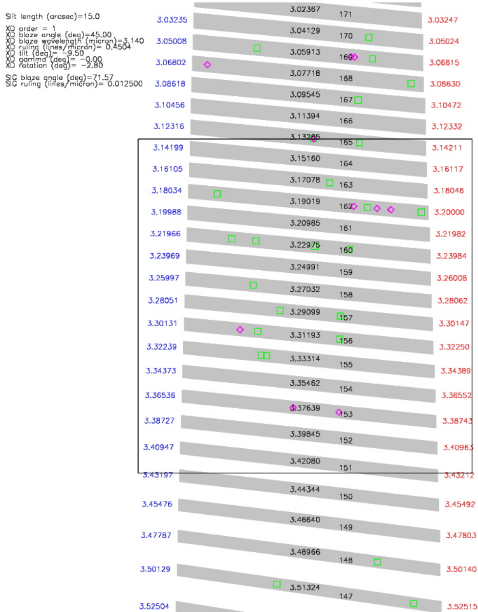
Figure 7. Exposure L3 (see Table 5), slit length 15", 450 line per mm grating. The box indicates the H2RG array.
