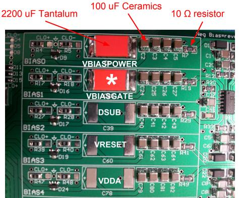
10  $\Omega$  resistor used on other channels for commonality since impact was minor. Only VBIASGATE requires low value resistor. If too large, there is a long ramp at beginning of readout due to channel output drawing a different current and the long time constant to reach steady state.
