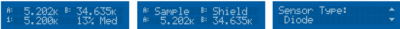
FIGURE 1-3 Displays showing two input/output display with labels, custom display with labels and the intuitive menu structure
