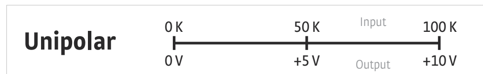
FIGURE 5-5 Output with polarity parameter set to unipolar
