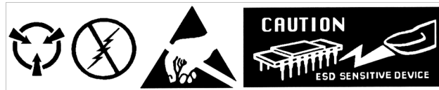
FIGURE 8-8 Symbols indicating ESD sensitivity
