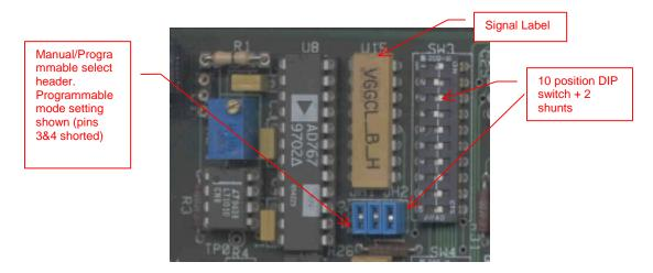
input 10 position DIP switch plus 2 headers that connect to the 12bit input of the DAC. There is also a Manual/Programmable Selection Header. If the header is configured for Manual control (pins 1&2 shunted) then
