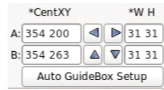
Figure 3-10. Arrows are used to fine-tune the position of the off-slit guide boxes.
