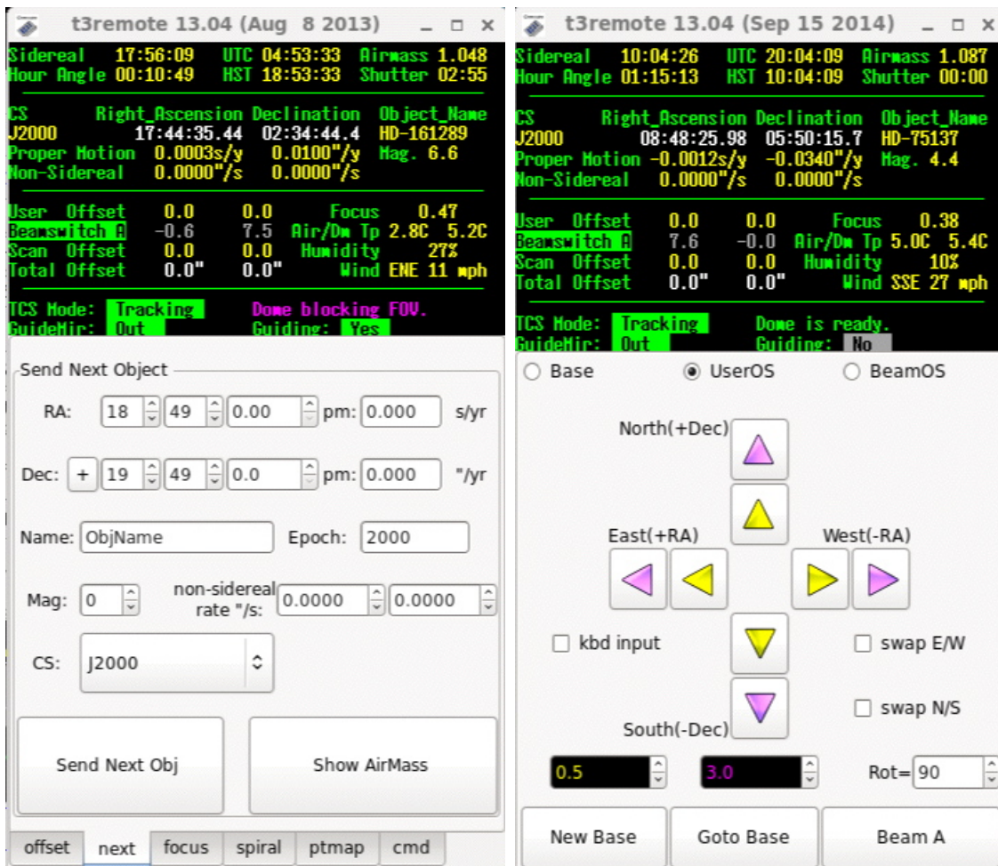
Figure 3-4. T3 remote TCS widget. Left - next panel to send object coordinates to the TO. Right - offset paddle panel for manual guiding. Set Rot to the position angle of the SpeX rotator to turn east-west and north-south on the paddle to horizontal and vertical in GDV.
