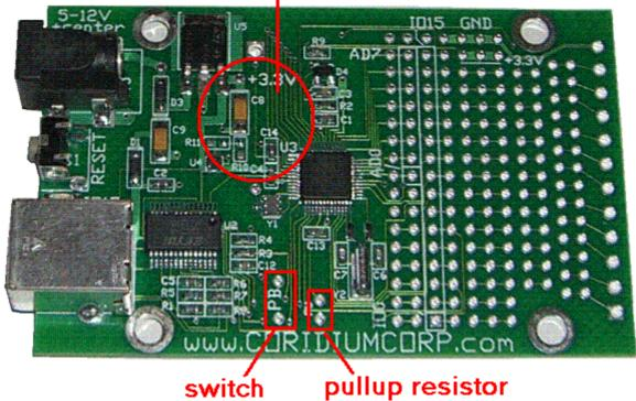
A push button switch and pullup resistor can also be mounted (connected to IO(2)). The optional battery for the real time clock (Panasonic ML2020) can be mounted on the back of the PCB. The VL2020/HFN will also work, though it is more expensive and has less power.
