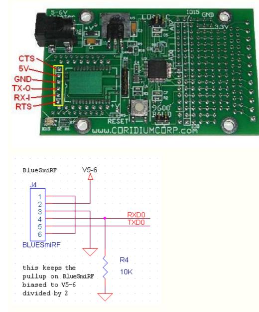
Shown below is one orientation with the BlueSMiRF mounted below the ARMmite-
