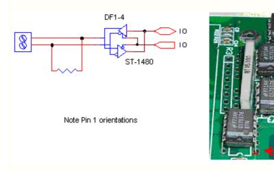
suggested components Bourns 4600 Isolated SIP resistor
