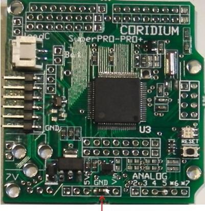
add ferrite bead (2200 ohm 50 mA 0603 or equivalent )
