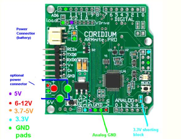
The 3.3V regulator can supply 50 mA, with most being used by the LPC2103. The 3.3V connection next to
