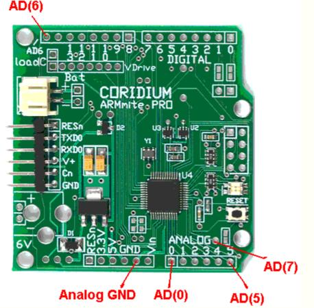
Picture is for the Rev 3 production board. On the Rev 1, AD(7) is available on a via next to AD(5).
