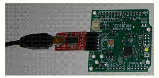
USB dongle from **Sparkfun** shown. Connect USB Cable to Computer
