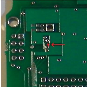
Then connect digital GND to analog GND using a ferrite bead, a convenient place to do this is on the front side as shown below.
