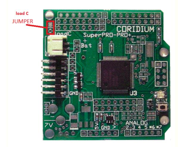
An alternative is to use a 2 pin header with a shorting block (pictured below)
