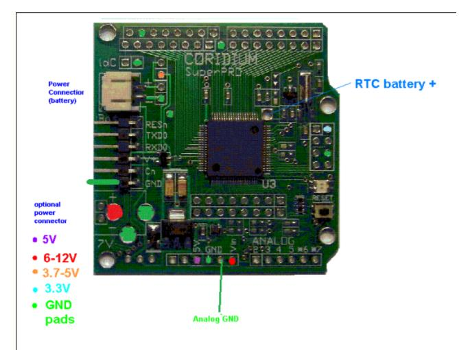
The 3.3V regulator can supply 50 mA, with most being used by the LPC2103. The 3.3V connection next to RESn on the lower power connector is only connected if the shorting pads are shorted (NOT the factory default).
