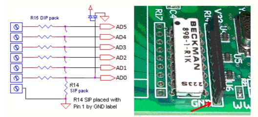
load R15 DIP resistor and R14 SIP with appropriate values
