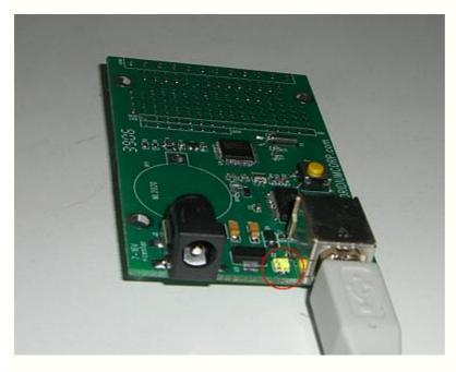
The Eval PCB or the ARMmite will be powered from the USB bus. It may also be connected to a 5-12V DC power source simultaneously.
