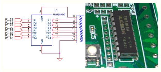
This driver can sink a surge current of 500mA upto 50V, this driver is a ULN2803 .
