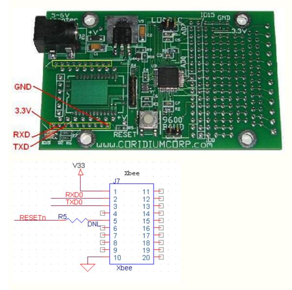
Shown below is the orientation with the Xbee module mounted on the ARMmite, using two 10 pin receptacles soldered into the ARMmite-
