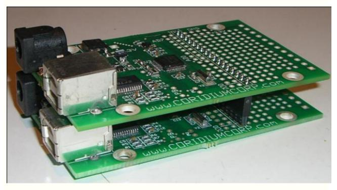
The ARMmite is a flexible solution to capture the logic state of your project. The ability to program the control of sampling in BASIC can be a powerful tool. Using a second ARMmite means that the timing of your code will not be affected when using LogicScope.
