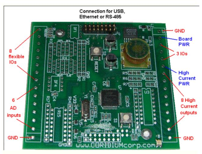
picture shown without screw terminals for clarity
