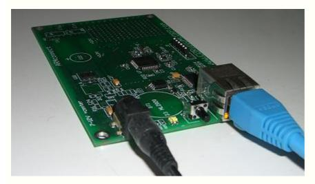
You should see a green LED connect light on the lower left side of the ethernet cable indicate a connection was made. Also your hub normally has a similar type of connection indicator. There should also be some traffic indicated on the right side as the ARMweb looks for a DHCP.
