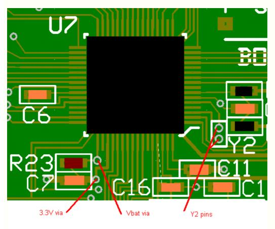
To connect a battery, remove R23, and use the Vbat via to connect, a resistor-Schottky diode-battery connection (suggested schematic below)
