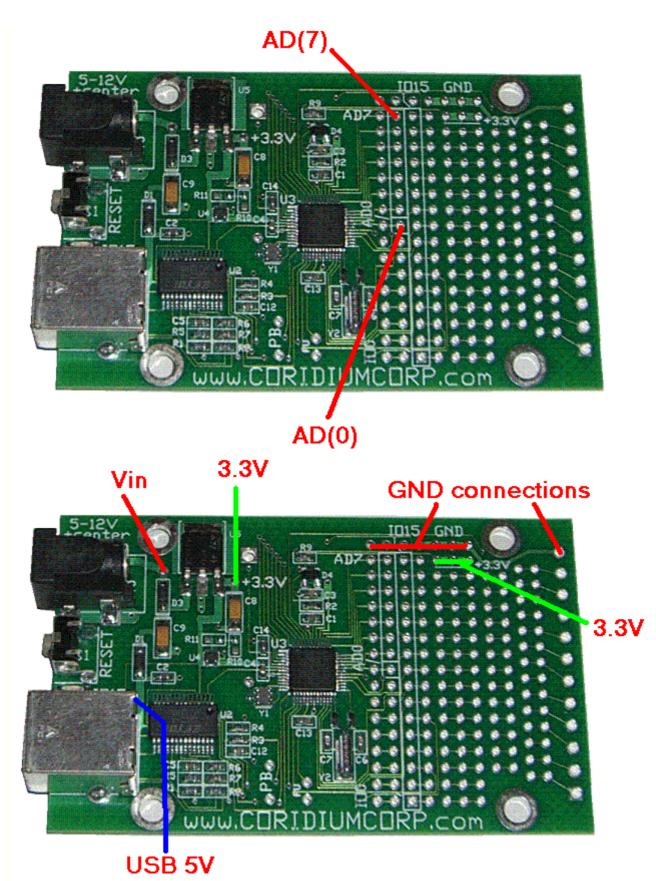
When USB power is not used, a 5-12V supply is required. If 5V is required for some portion of your circuit, it is suggested that a regulated 5V supply be used for input power. These are available from **SparkFun**.
