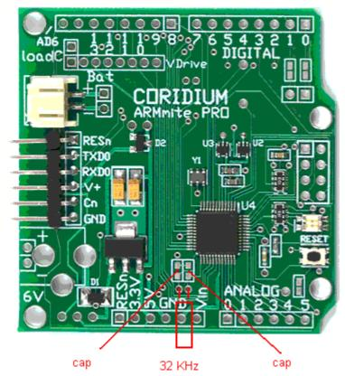
The crystal should be a 32.768 KHz can type, and depending on the rating the capacitors are 0603 size 18-27pF.
