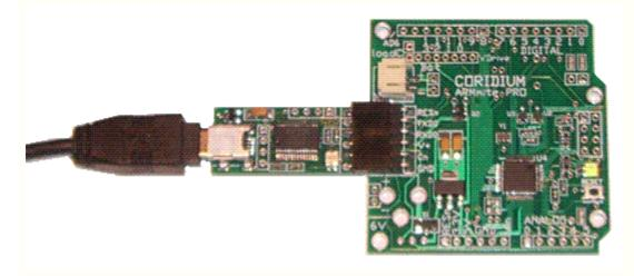
The ARMmite PRO will be powered from the USB bus, when using either the Coridium Dongle or the FTDI 5V cable. It may also be connected to a 6-7V DC power source simultaneously.
