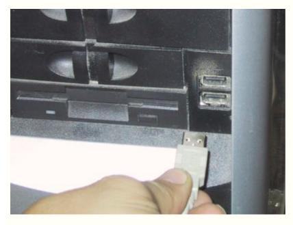
Locate the USB jack on your computer and plug the other end of the cable into it.
