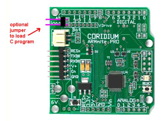
An alternative is to use a 2 pin header with a shorting block (pictured below)
