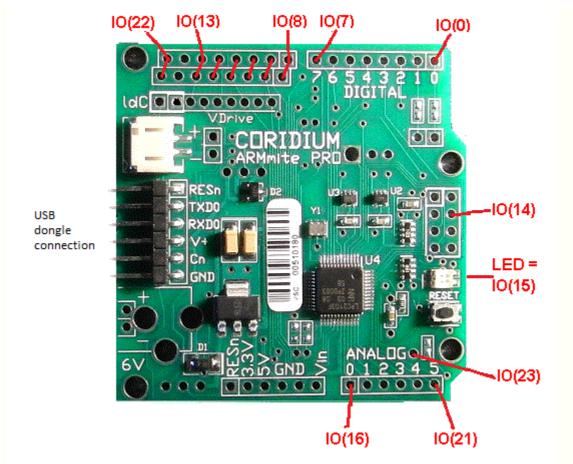
The major change for rev 4 is to add a parallel connection for the 8 IOs IO(8)-IO(13), GND and IO(22) that is on 0.1" centers in relation to the other connections.
