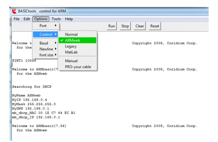
Again, if you don't see the LEDs or this display, check your power connections (you should see at least 6V of the + side marked on C23, and 3.3V as marked in the prototype area), check your com connections (details in Troubleshooting section ).
