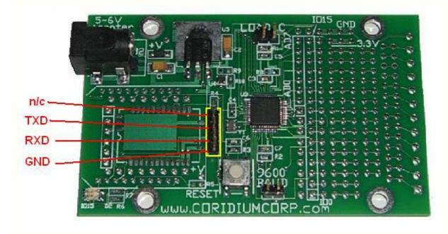
Additional pins may be wired up to the USB breakout board, so that it will work identically with the original ARMmite. In this case 5V from the USB will power the board. But when that connection is made a power supply should NOT be connected.
