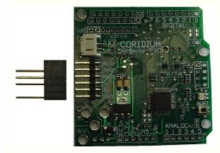
The above shows both RESET and BOOT signals disconnected.
