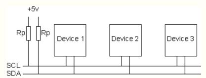
The value of the resistors should be from 1.8K (1800 ohms) to 4.7k (4700 ohms). It depends on the length of the I2C bus, the longer the bus, the smaller value should be used. If the value is too large, the rise time of the signals will be too slow and the bus may not work properly. If the resistors are missing, the SCL and SDA lines will always be low - nearly 0 volts - and the I2C bus will not work.
