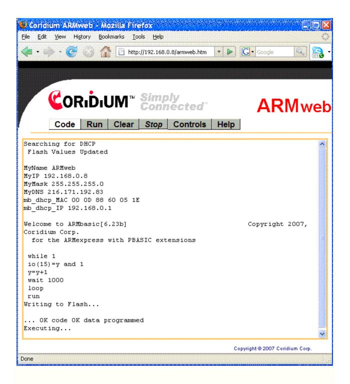
WHILE 1 IO(15) = Y AND 1 'Flash the LED Y = Y + 1 WAIT 1000 LOOP RUN
