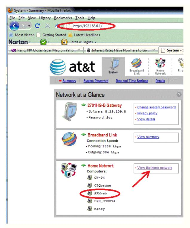
Most DHCP servers will list client machines which have been assigned an IP address. This 2wire server indicates it on the details view of the home network, and details for the device
