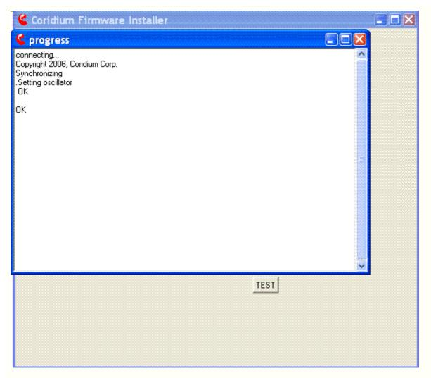
If this does not pass, then you **cannot** go on to the next step. You must verify your connections, choice of COM port, and whether you are driving P0.14 low while driving RST on the LCP2xxx low, and then releasing it. These would be the same steps you use to program any hex file with a program like FlashMagic. Refer to the documents that came with your PCB.
