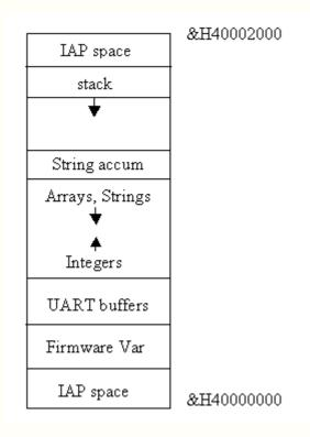
Local variables for FUNCTIONs and SUBs are allocated from global memory. This allows for a smaller stack size and faster calls to FUNCTIONs and SUBs. The ARMmite has only 8K total and has no stack overflow checking.
