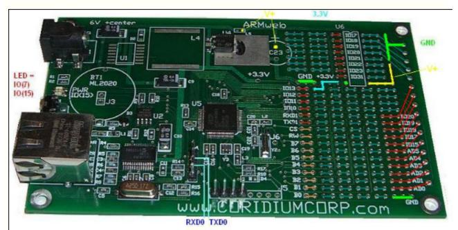
U6 has duplicate connections for IO(17)-IO(20). U6 is designed to accept a ULN2803.
