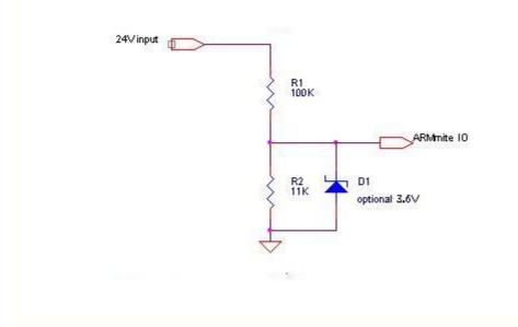
The resistors can be varied to handle different voltages. If the voltage to be sensed is susceptible to large spikes a 3V Zener diode can be connected in parallel with R2 to further protect the ARMmite IO.
