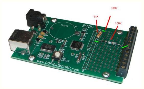
This resistor divider divides the 24V by 10 and also limits the current if that 24V goes higher. The circuit below shows schematically the connection that was made.
