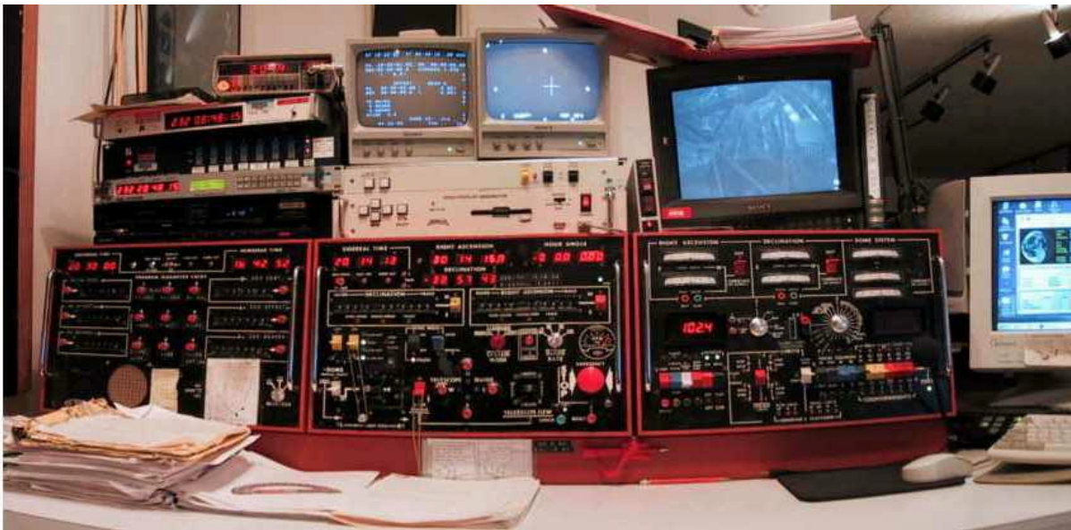
Figure 2. Photo of the Master Control Console (MCC) as viewed by the Telescope Operator. Several other workstations for star catalogs, tip-tilt guider, and network services are not shown.
