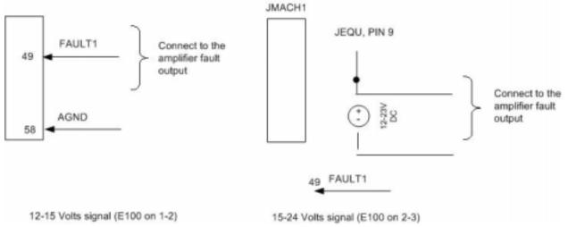
Some amplifiers share the fault output with the enable\disable status output. In this case a special PLC code must be written with the following sequence:
