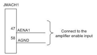
This signal could be either sinking or sourcing as determined by chips U37. (See jumpers E100-E102.) For 24V operation, E100 must connect pins 2-3 and a separate power supply must be brought on pins 9-7 of the J9 JEQU connector. The polarity of the signal is controlled by jumpers E17A to E17D. The default is low-true (conducting) enable. Also the amplifier enable signal could be manually controlled by setting Ix00=0 and using the suggested definition of the Mx14 variable.
