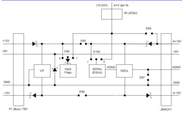
**E85, E87, E88: Analog Circuit Isolation Control** – These jumpers control whether the analog circuitry on the PMAC is isolated from the digital circuitry, or electrically tied to it. In the default configuration, these jumpers are off, keeping the circuits isolated from each other (provided separate isolated supplies are used).
