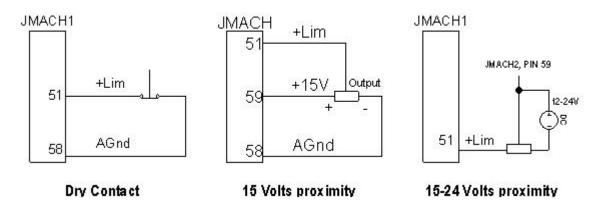
Jumper E89, E90 and E100 must be set appropriately for the type of sensor used.
