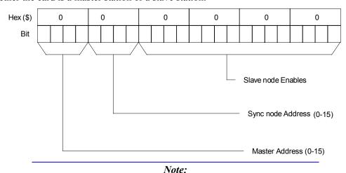
On prototype PMAC2 boards that did not support multi-master MACRO rings, I996 contained only bits 0-15.
