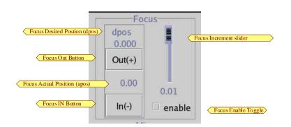
The Focus control are located on the MCC2 GUI Tab. Details are located in MCC/Details/FIOC. The ic/fio c/focus.c program controls the focus control.
