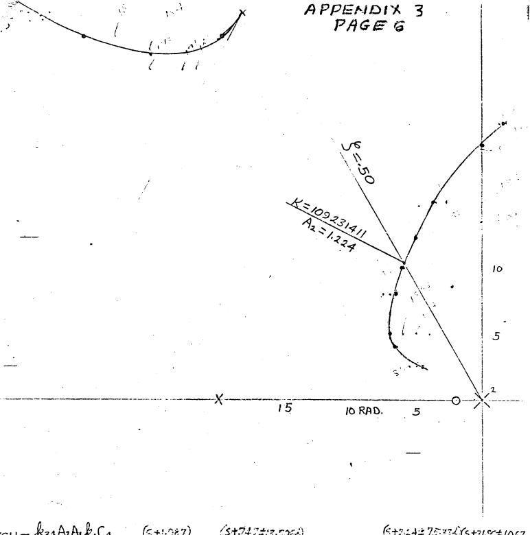
$(GH = \frac{k_{34}A_{2}A_{1}k_{1}C_{4}}{J_{3}J_{4}} = \frac{(S+1.987)}{(S+19.87)S^{2}(S+2316)(S+31.92\pm10.67)} = \frac{k_{34}A_{2}A_{1}k_{1}C_{4}}{(S+19.87)S^{2}(S+2316)(S+31.92\pm13.274.2)(S+18.08\pm29.372)(S+2.242\pm75.75)k_{1}S+185\pm475.75}$
