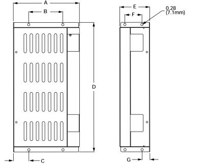
D/E - SIZE FILTER ENCLOSURE DIM. INCHES mm. A 7.75 196.9 B 4.00 101.6 C 1.81 46.0 D 15.25 387.4 E 3.52 89.4 F 2.00 50.8 G .92 23.3
