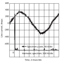
PWM Converter Input Drive - 4 kHz PWM
