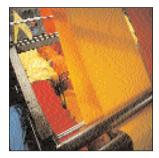
Winders / Unwind Stands - Baldor Line Regen AC drives control roll tightness, tension, stretch or draw of the material in web processing systems. They comply with IEEE-519 for THD to protect other on-line equipment including other variable speed drives from harmonic disturbances. Web processing systems are found in paper, textiles, wire, printing and metal manufacturing industries.
